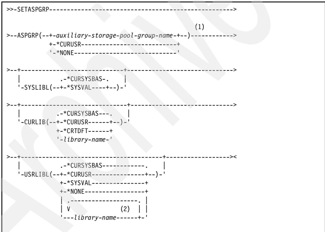
Figure D-4 SETASPGRP (Set ASP Group) syntax diagram
